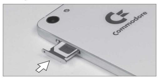
Be careful to never force the tray during this operation. You just need to push the tray back in its bay and, when it's near to be closed, slide your finger up and down on its side surface without using any strenght.
