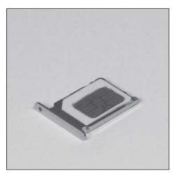
4 You can also use the second side of the tray to install a secondary nano-SIM card (dual SIM option) OR to add a memory expansion card (MicroSD, up to 64GB).
